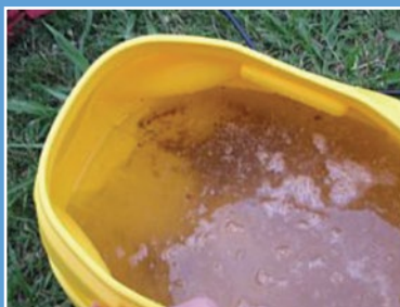
Water from an untreated drain pan
